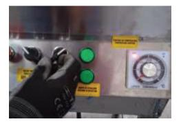
Turn the temperature control switch ON
