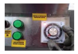
The pyrometer OFF indicator will turn on in the zero position.
