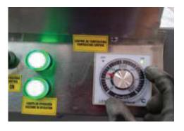
Turn the pyrometer to 140-160°C, and the indicators of the equipment in operation will turn on.
